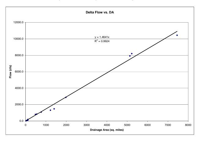
Figure 4. Delta Drainage Area to Flow Comparison
