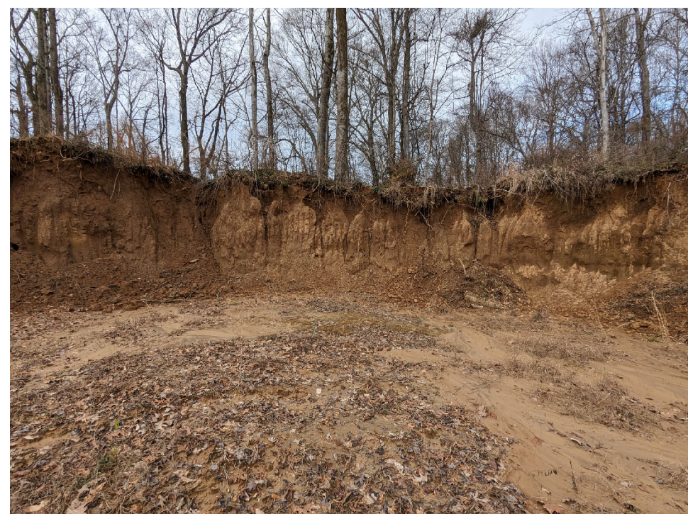
Thick deposit of Pleistocene loess exposed in the high wall of a recent borrow pit used for fill dirt in Section 36, Township 9 North, Range 3 West.
