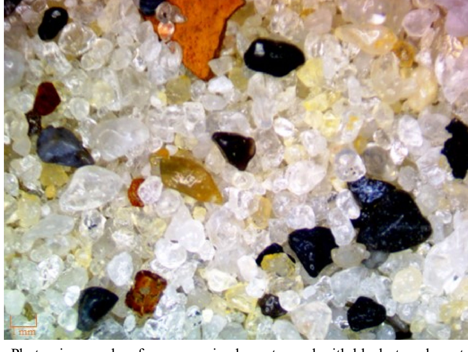
Photomicrographs of coarse-grained quartz sand with black, translucent, angular, and unweathered chert grains from the upper Oligocene Catahoula Formation recovered from a depth interval of 200-210 feet in MGS Providence Hill Farm #1 stratigraphic test hole B-0034 drilled on April 4, 2023 in Section 21, Township 7 North, Range 2 West. Scale in millimeters.
