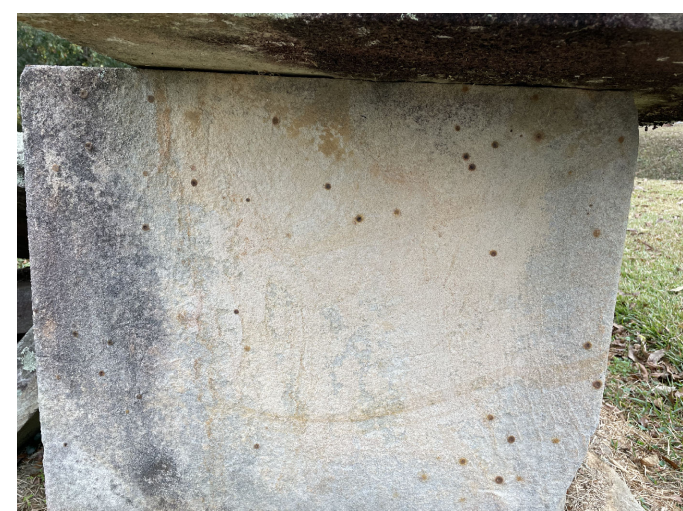
Pyrite weathering and crossbedding in box-grave monuments in the old Raymond Cemetery made of Catahoula sandstone quarried at Mississippi Springs. Photographed on November 18, 2021.
