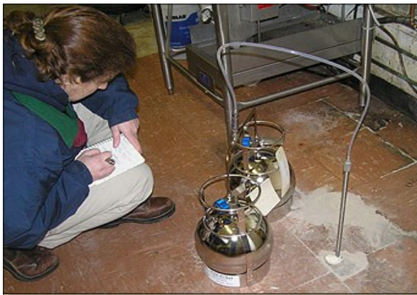
An example of a sub-slab vapor sampling.
