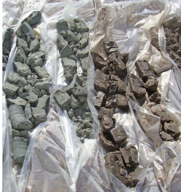
Figure 9. Color contrast between the light blue-gray Moodys Branch Formation sand on left and chocolate brown Cockfield Formation clay on the right.
