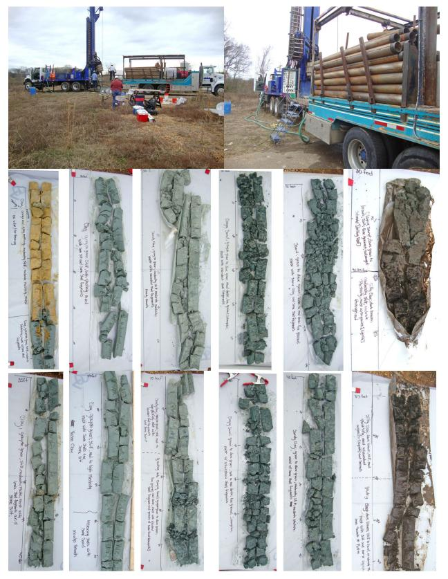
Figure 7. Large Sonic drill rig (top) and core (bottom) taken at the Southeastern Wood Preserving Supterfund site in Canton, Mississippi, on January 8, 2013. From left to right are core intervals 30-40, 40-50, 50-60, 60-70,70-80, and 80-90. The top of the Moodys Branch Formation is at 57.3 feet and the bottom at 81.9 feet. Pictures from *Mississippi Environmental Geology*, 2018, p. 228.
