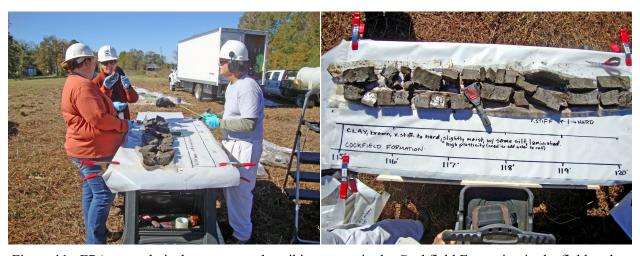
Figure 11. EPA geotechnical contractors describing a core in the Cockfield Formation in the field at the Southeastern Wood Preserving Superfund site on November 8, 2012.
