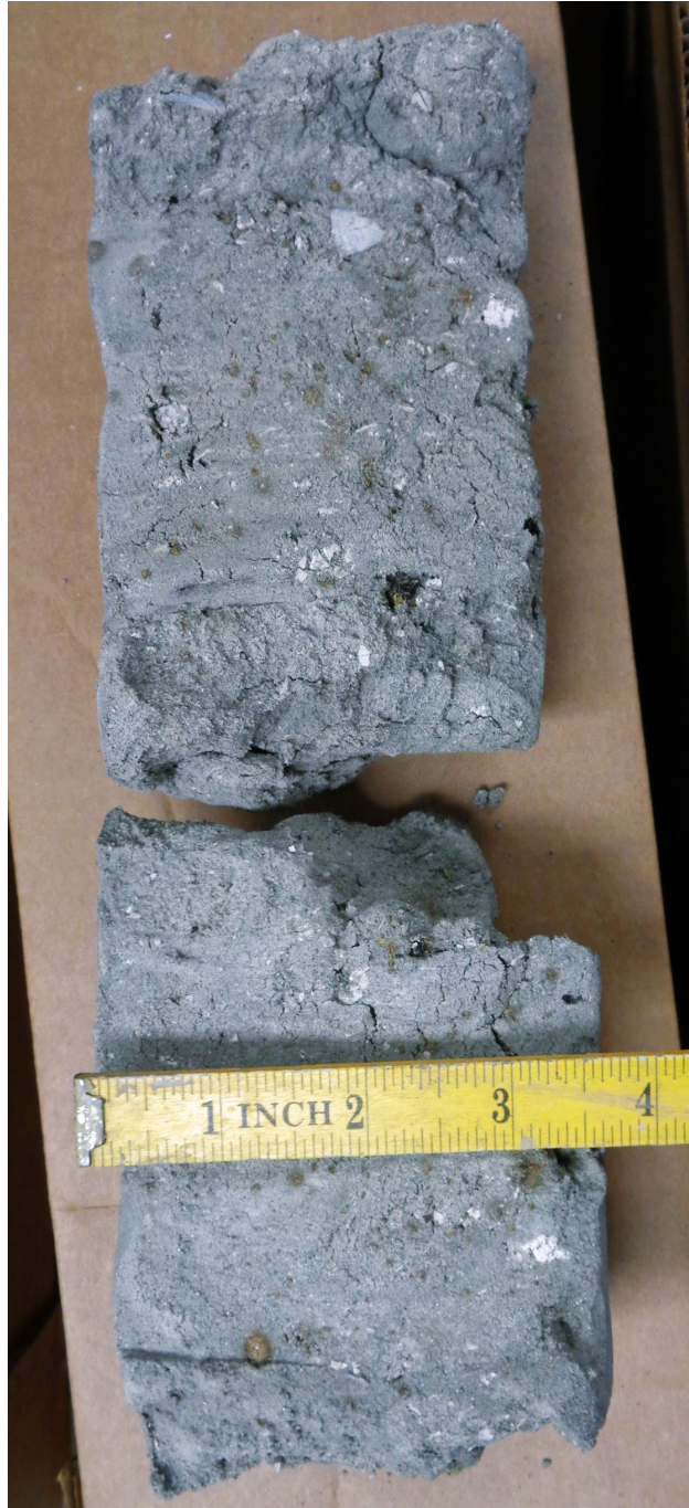
Figure 12. This boxed 3.5-inch diameter core half is from the upper clay-rich part of the Moodys Branch Formation at the Southeastern Wood Preserving Superfund Site at Canton, Mississippi. It is stored in MDEQ Office of Geology's Core and Sample Library in Jackson, Mississippi.
