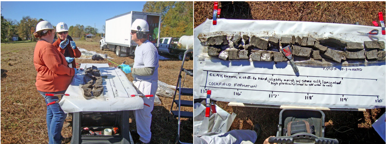
Figure 11. EPA geotechnical contractors describing a core in the Cockfield Formation in the field at the Southeastern Wood Preserving Superfund site on November 8, 2012.
