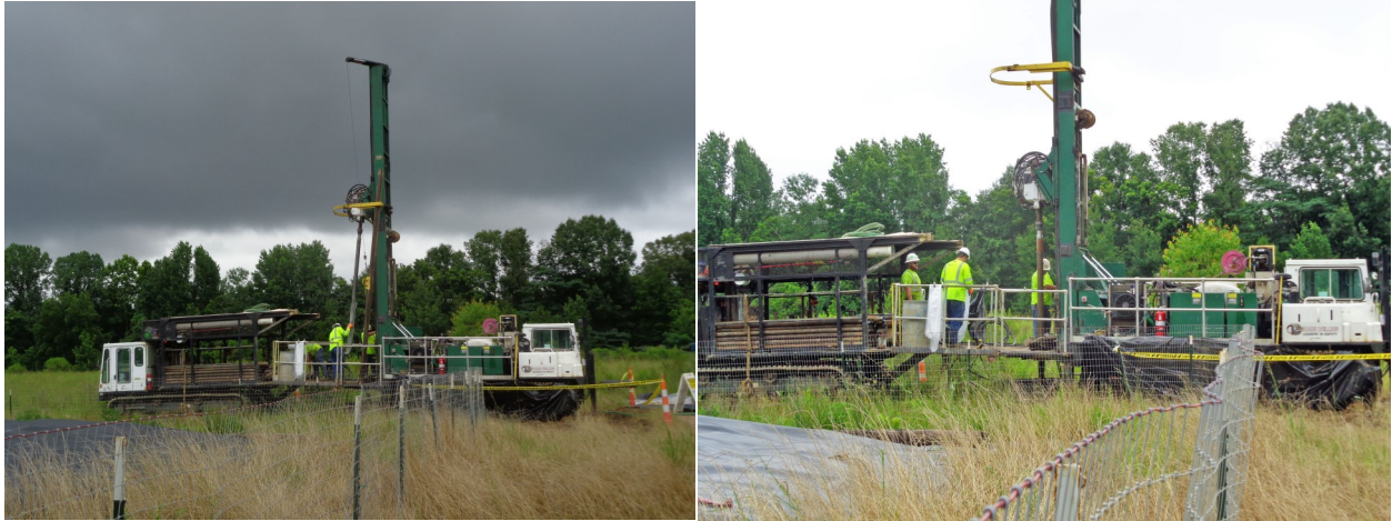
Figure 4. Sonic drilling rig coring at the Southeastern Wood Preserving Superfund Site on June 19, 2017, in stormy and fair weather.
