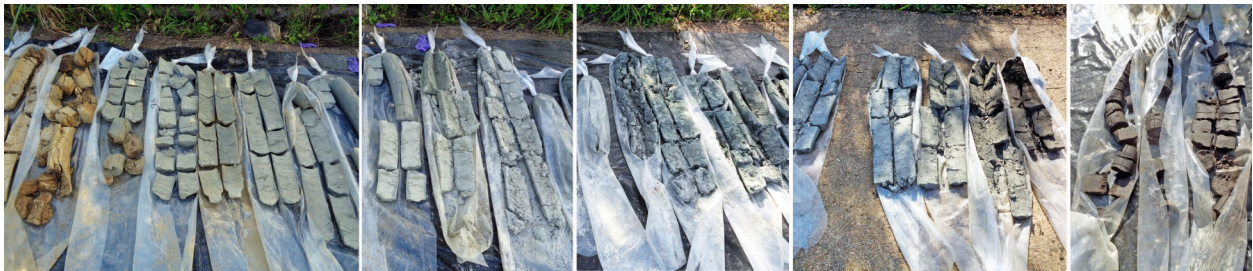
Figure 5. The core, from left to right, penetrated the brown weathered Yazoo Clay, the gray unweathered Yazoo Clay (frame 1), the sandy Moodys Branch Formation (2-4), and the Cockfield Formation (4-5) with a lignite seam at the top (4, last core at right).
