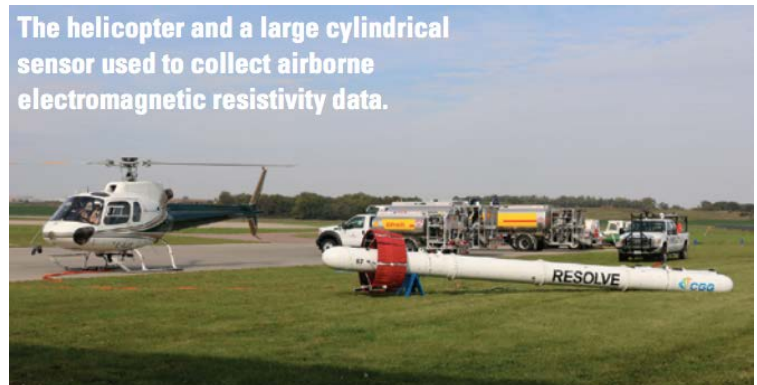
Diagram (left) showing airborne geophysical survey layout, instruments and subsurface rock layers. Picture (right) showing the RESOLVE electromagnetic sounding equipment used recently in South Dakota.
