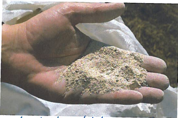
Amendment material - used to treat soil - 3% by volume
