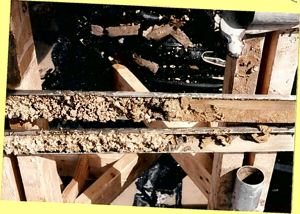
Photo 5. Split spoon sample from the third boring taken on school property. Free product can be seen on the right end of the sample
