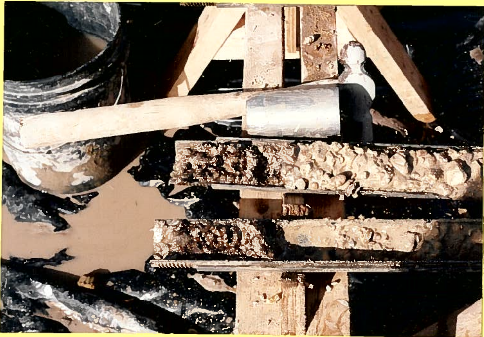
Photo 5. Split spoon sample from the third boring taken on school property. Free product can be seen on the right end of the sample
