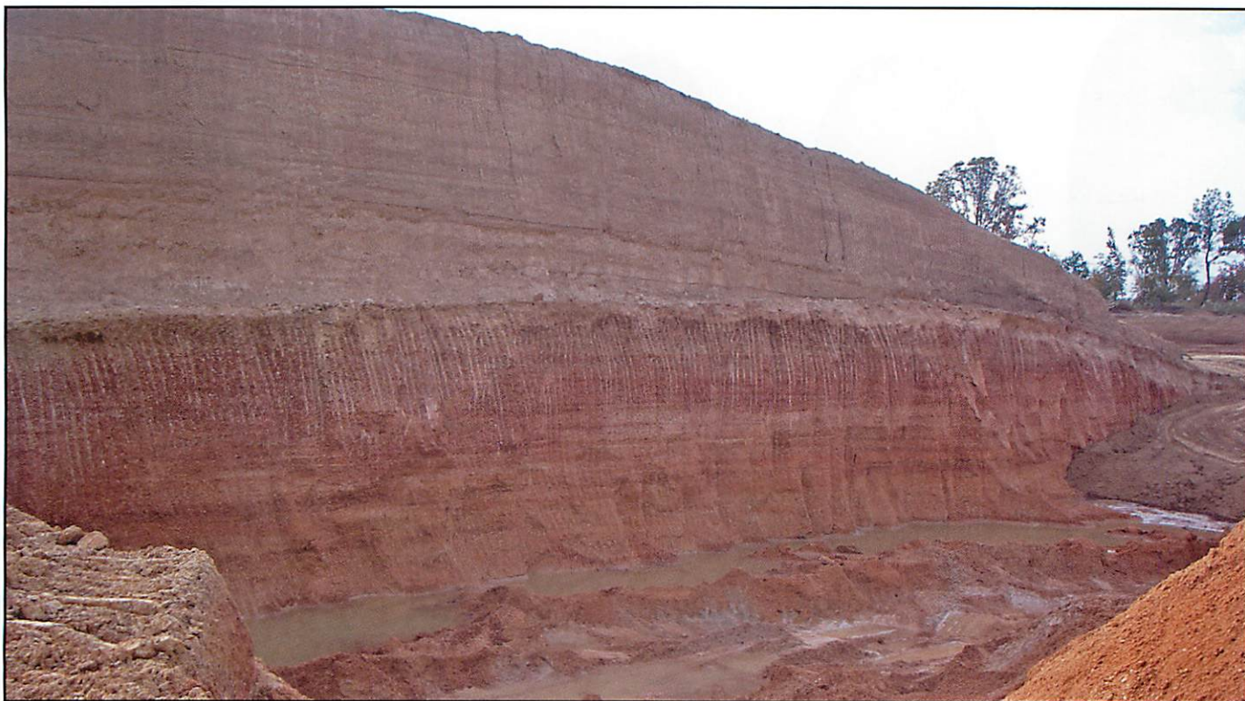
Figure 2. Highwall exposed at the Hammett Gravel Company Zieglerville pit in Yazoo County. The upper half of the highwall consists of a 25-foot-thick section of loess. A brown ancient soil (paleosol) can be seen at the loess-gravel contact. The lower 25 feet of the highwall contains pre-loess gravel. The water table can be seen in the bottom of the pit, below which is more gravel. Picture was taken on November 9, 2007.
