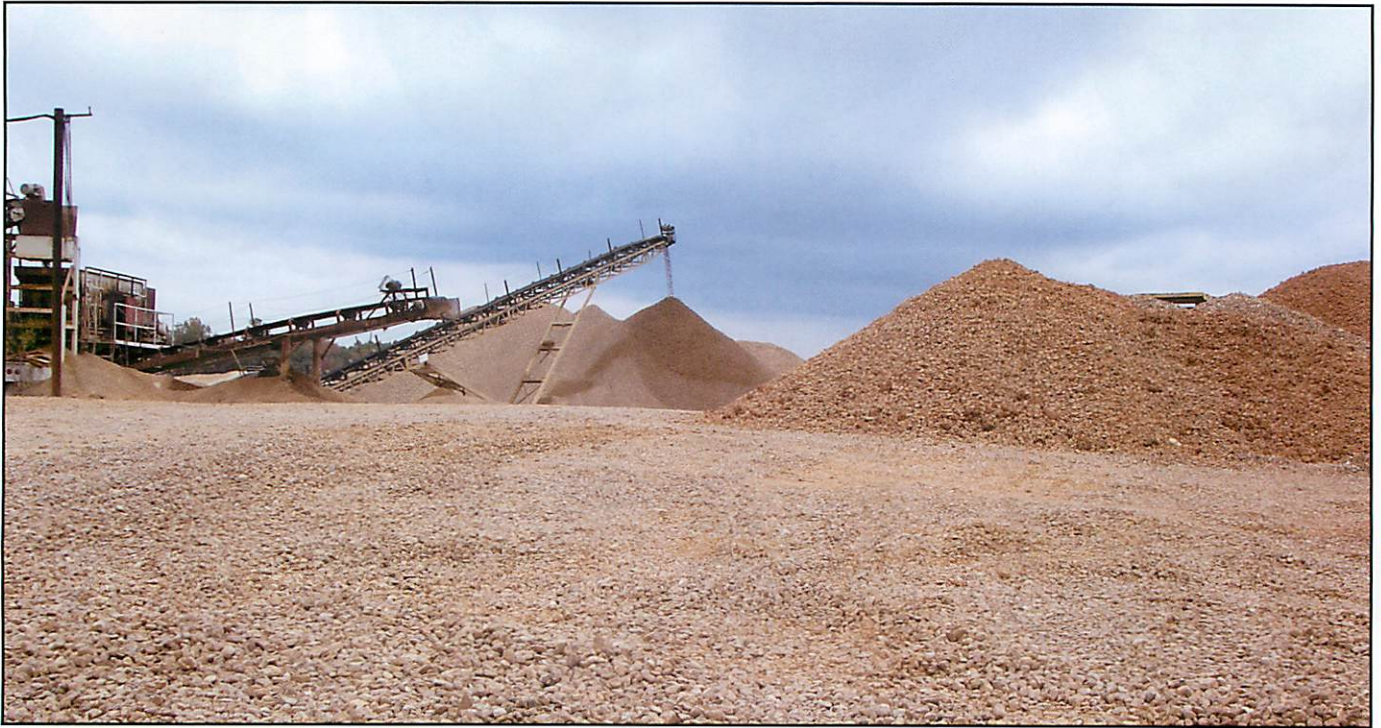
Figure 3. Gravel washing operation located at the Zieglerville pit in Yazoo County. Gravel is transported to this site by a conveyer belt from the active mine, which is more than a mile away. Picture was taken on November 9, 2007
