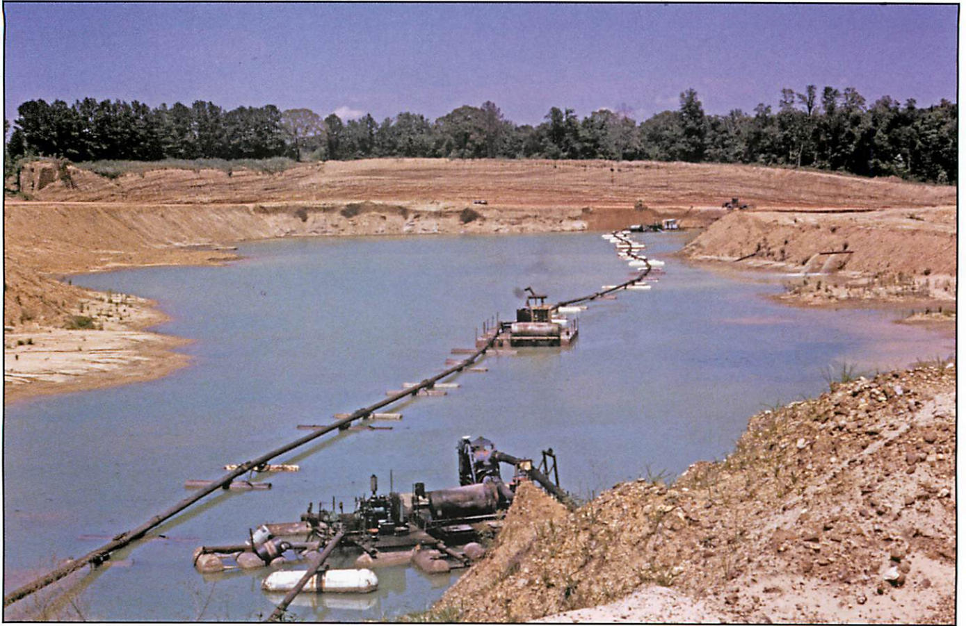
Figure 7. Gravel dredging in pre-loess gravels below the water table at the Hammett pit in Yazoo County. Picture was taken on May 5, 2004.
