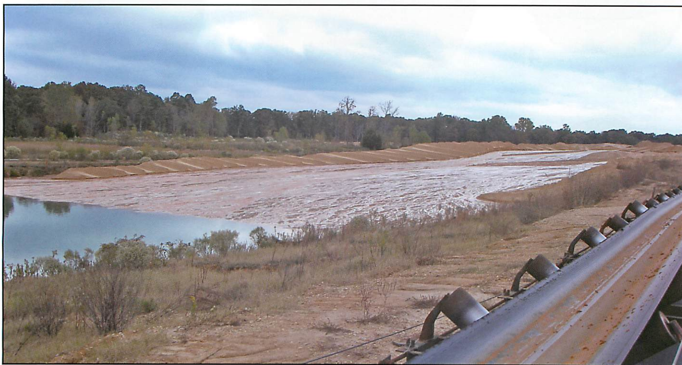
Figure 4. Sand draining from gravel wash operation forms a delta at the head of a containment lake. The conveyer belt that transports the gravel to the gravel wash is at the lower right. Picture was taken on November 9, 2007.
