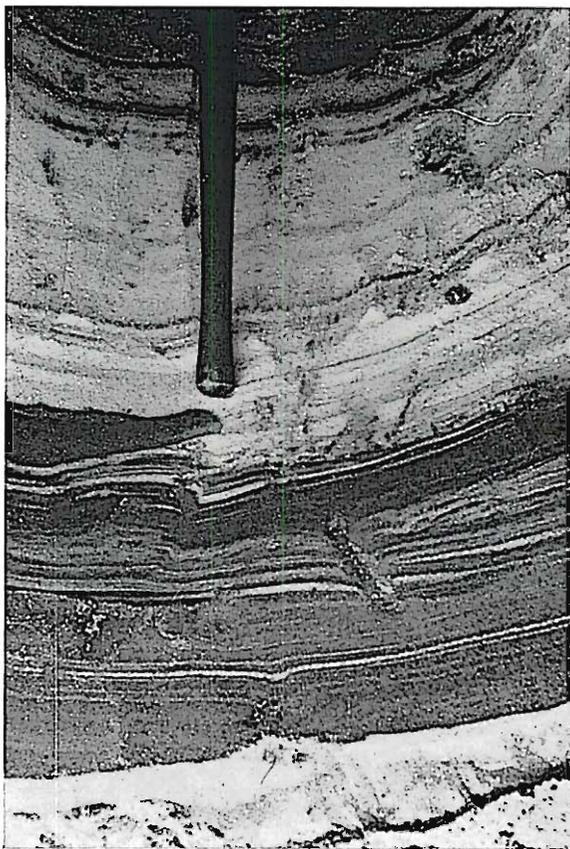
Figure 21.—Intertongued beds of "heavies," Gulf side of West Ship Island, due south of "6 sec. flashing beacon," at hand auger hole 6. The concentrate tested 52 percent "heavies." Photo by W. S. Moore, July 1959.
