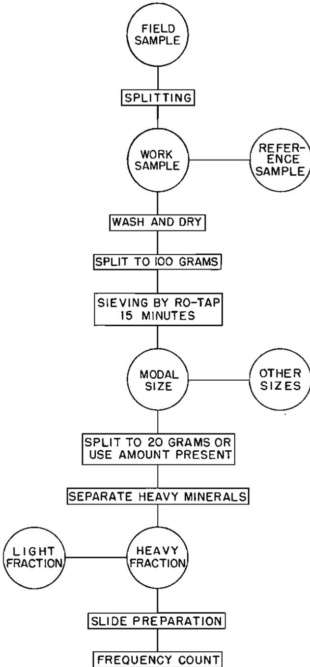
Figure 25.—Flow sheet for laboratory procedure.
