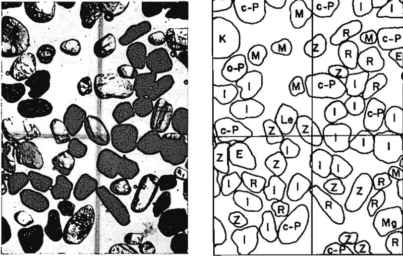
Figure 26.—Photomicrograph (left) of West Ship Island "heavies." Total magnification 43.2; uncrossed prisms; Ansco Veraspan fine grain film, speed 40. Photographed by Johnson and Smith, July 24, 1961. Tracing from film on the right. Mineral grains designated thus: E epidote, I ilmenite, K kyanite, Le leucoxene, M monazite, Mg magnetite, R rutile, c-P clino-pyroxene, o-P ortho-pyroxene, and Z zircon.
