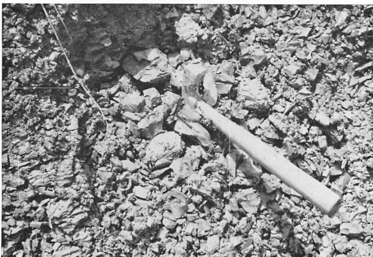
Figure 6.—Slightly weathered Porters Creek clay exposed in a cut (NW.¼, SE.¼, Sec.24, T.12 S., R.1 E.) of a road on the lower south slope of the Skuna River valley 2.9 miles east-northeast of State Highway 341. July 21, 1961.
