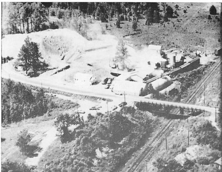
Figure 20.—Aberdeen plant of American Colloid Company on Aberdeen Branch of Illinois Central Railroad Company, Monroe County. "Panther Creek" Eutaw bentonite is produced as foundry bonding clay. Photo American Colloid Company, 1959.
