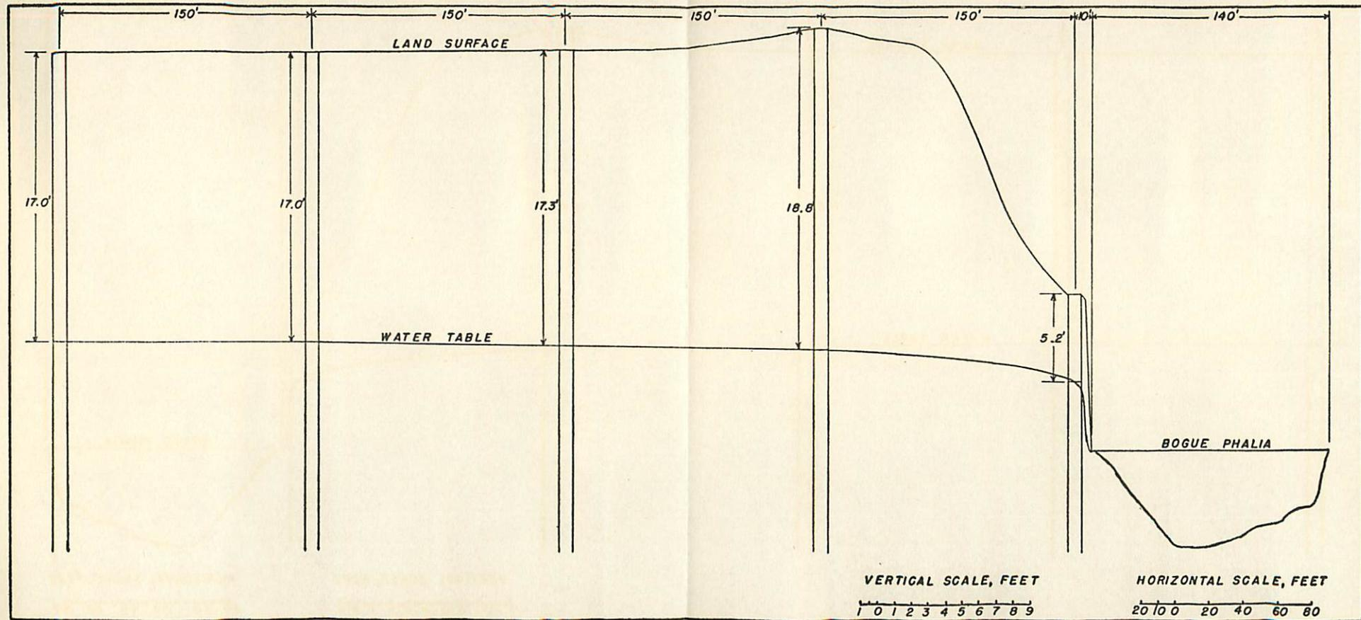
Plate 2.—Cross-section of Bogue Phalia and test holes at right angle to Bogue Phalia.
