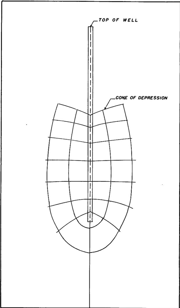
Plate 3.—Flow net of test well.
