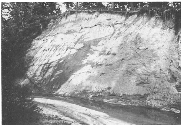
Figure 10.—Upper Zilpha Clayey silts overlain unconformably by Citronelle gravel. Here, test hole H123 was drilled to a depth of 120.5 feet. September, 1940.
