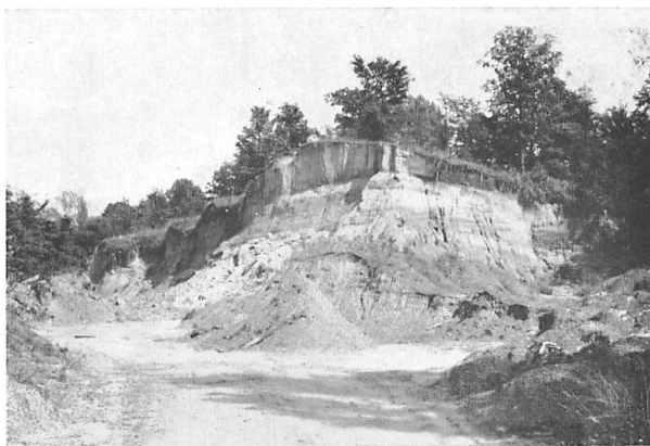
Figure 5. —Fox and Guthrie gravel pit, 7 miles north of Charleston. The face of the pit shows 38 feet of gravel overlain by 18 feet of loess. April, 1941.
