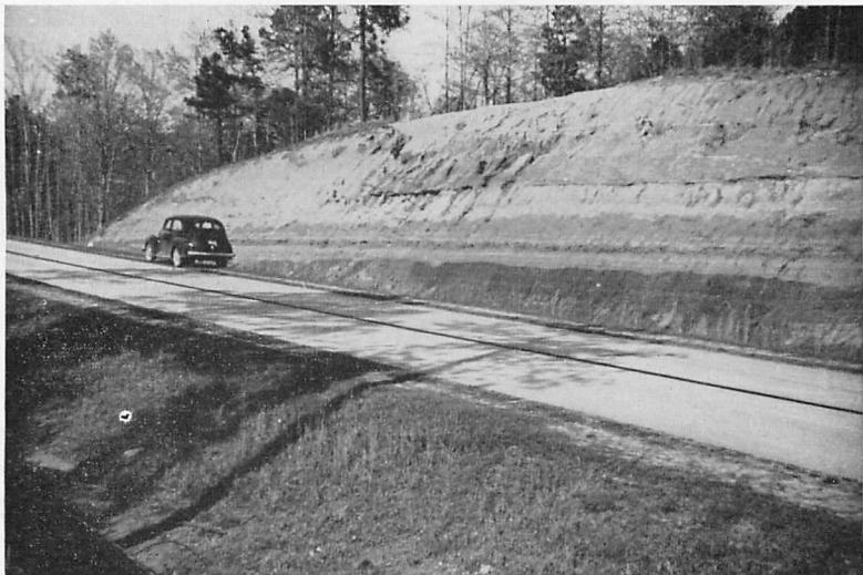
Figure 19.—Cross-bedded Cockfield sands over lignitic, silty shales of Gordon Creek member. Cut on Highway U. S. 11, 0.1 mile east of Wautubbee Station, Clarke County.
