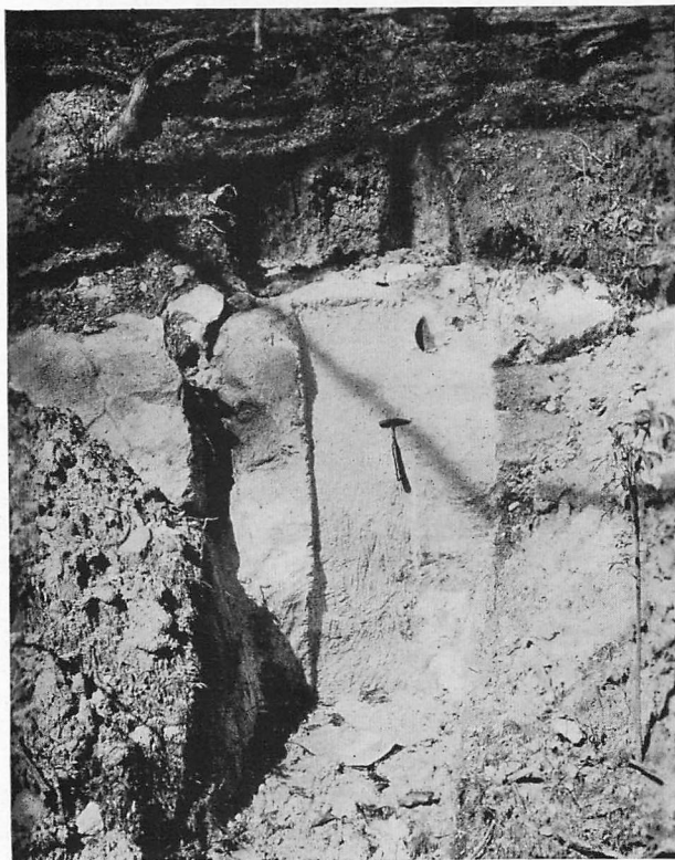
Figure 18.—Test hole 88, a trench exposing a seven-foot face of hard bauxitic clay on the property of the Fair Lumber Company (SE. \frac{1}{4} , NW. \frac{1}{4} , Sec. 22, T.14 N., R.14 E.). The sample for testing was taken from the channel in the middle of the picture.---March 24, 1938.
