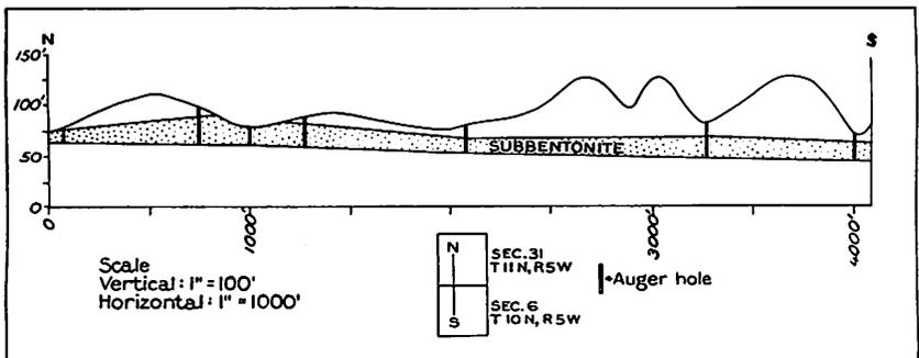
Figure 3.—Cross section of the deposit of sub-bentonite east of Matherville, Wayne County, Miss.
