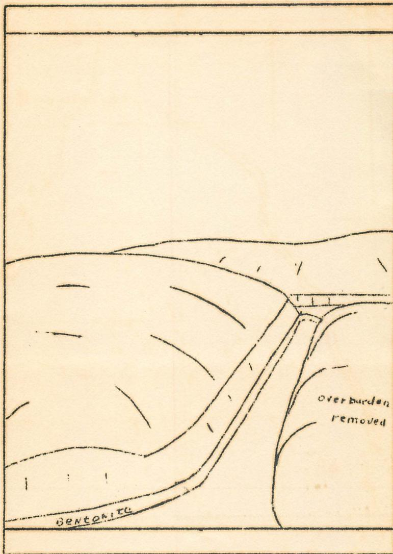
Showing relation of bentonite to overburden in bentonite mine
