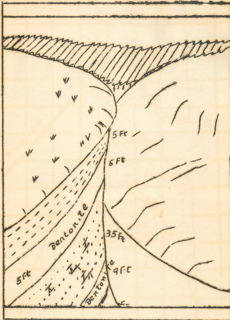
Showing relation of two bentonitic beds in the side of a cliff 55 feet high on Panther Creek, in Sec.26, T15S, R7E, Monroe Co.
