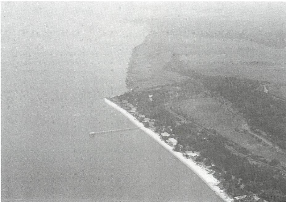
Figure 15. Shoreline offset caused by groin construction at the west end of Belle Fontaine Beach.
