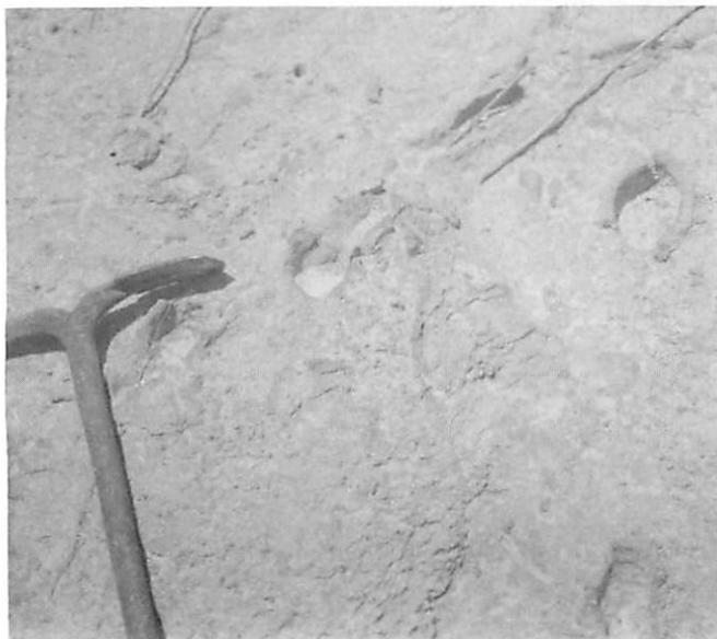
Figure 50 — Low elevation terrace material in outcrop. Note root structures and mottled appearance of massively bedded sand. Location: SE/4, SE/4, SW/4, Sec. 17, T.6N., R.10E.
