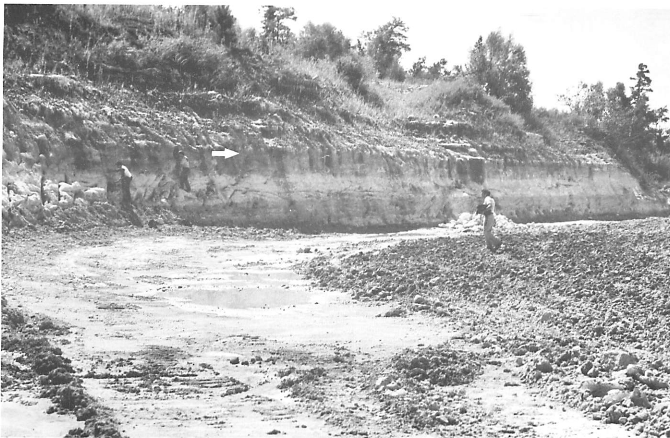
Figure 10 — Marianna and Glendon limestones at the Smith County Lime Plant quarry (MGS locality 92) in the NW/4, NE/4, Section 27, T. 2 N., R. 9 E., Smith County, Mississippi. The soft Marianna Limestone, which forms the vertical portion of the quarry wall in the background, is disked up (foreground) here and allowed to dry before its conversion into agricultural lime. The ledge-forming Glendon Limestone forms the upper slope of the quarry wall. The arrow marks the Marianna - Glendon contact. Gary S. Zumwalt is at right. Photograph taken on October 24, 1983.
