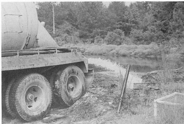
Figure 6.—Truck dumping salt water into an evaporation pit. Location is in Eucutta Oil Field, in NE/4, SE/4, NW/4, Sec. 6, T.9N., R.8W. August 1973.
