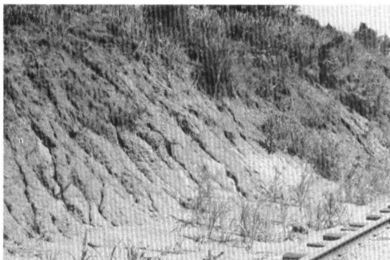
Figure 18.—Residuum overlying slightly weathered Glendon limestone along west bank of railroad cut in west Brandon. May 1, 1971.
