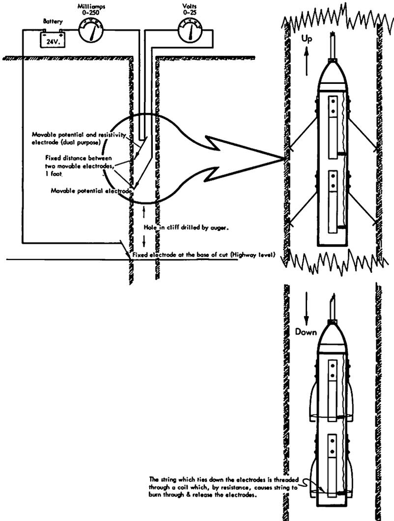
The string which ties down the electrodes is threaded through a coil which, by resistance, causes string to burn through & release the electrodes.
