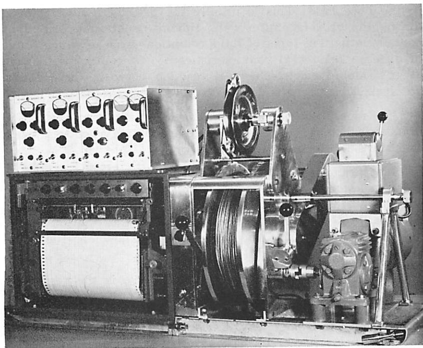
Figure 1.—Neltronic 2K Logger similar to the Survey's but equipped with additional panels that allow several more functions to be performed. The Survey logger is capable of making conventional two-curve electrical logs (self potential and resistivity) and gamma ray logs up to depths of 3,300 feet. The additional panels may be added as needed without modification of the instrument. Note electrical log tracing on chart. Photo provided by Neltronic Instrument Corporation.
