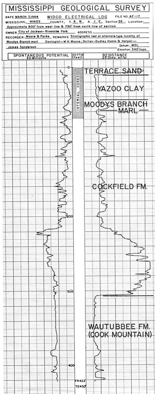
Figure 10.—Electrical log of the hole drilled to sample the lower Jackson Yazoo clay and Moodys Branch marl at Riverside Park at Jackson.
