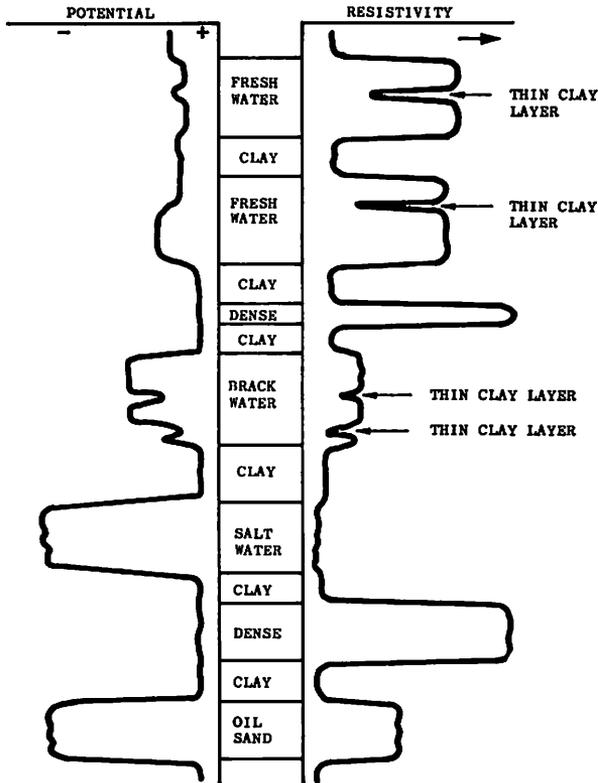
Figure 2.—Idealized electrical log. Note that the potential curve defines many of the boundaries of units and indicates the nature of many formations. Also, the resistivity curve shows that fresh water sands and dense formations have greater resistivity values than salt water sands, clays and shales. From the Widco Logger OPERATOR'S MANUAL published by Electro-Technical Laboratories.
