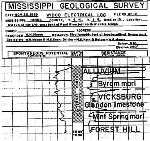
Figure 7.—Electrical log of the hole cored to sample the Vicksburg "group" near Byram.
