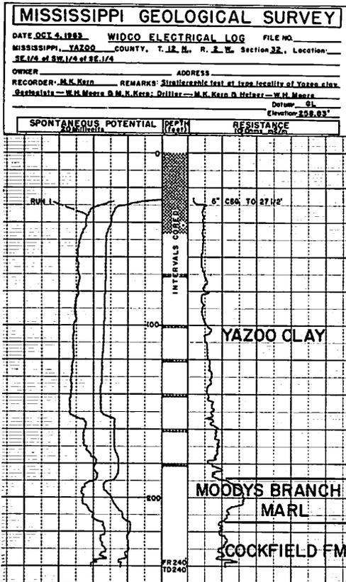
Figure 4.—Electrical log of the hole drilled to sample the Yazoo clay at Yazoo City.
