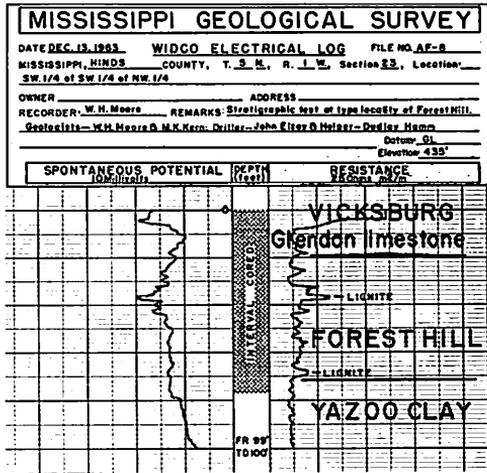
Figure 9.—Electrical log of hole drilled to determine the stratigraphic position and thickness of the Forest Hill sand at Forest Hill.
