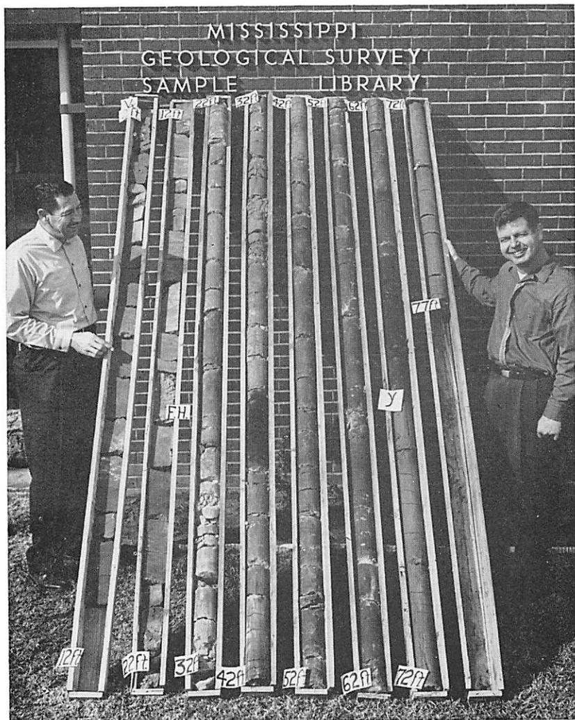
Figure 8.—Core taken at Forest Hill to sample the Forest Hill sand. Left to right and top to bottom — from Vx to F. H. is weathered Glendon limestone and marl; from F. H. to Y. is Forest Hill sand, silt, clay, and lignite; and from Y. to 77 ft. is uppermost Yazoo clay. Note two beds of lignite (dark-colored) in Forest Hill.
