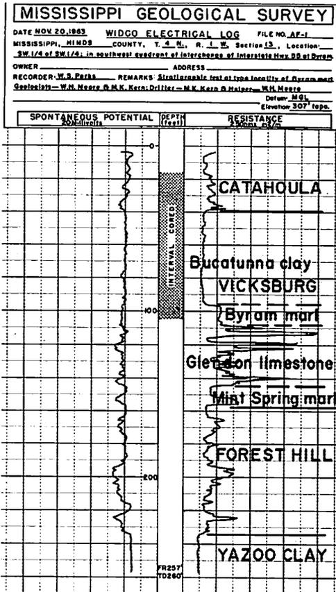
Figure 6.—Electrical log of the hole drilled to determine the stratigraphic position and the thickness of the Byram marl at Byram.
