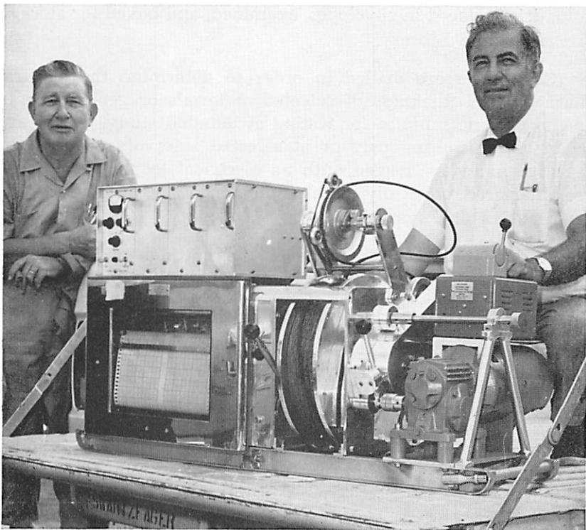
Figure 2.—Survey's new Neltronic 2K electrical logger capable of making conventional two-curve logs (self potential and resistance) and also gamma ray logs up to depths of 3,300 feet. Claude Sutherland photo. August 19, 1964.
