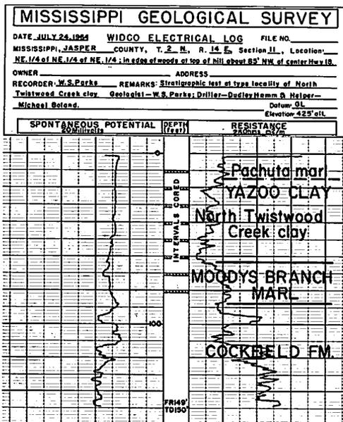
Figure 14.—Electrical log of the hole drilled to sample the North Twistwood Creek clay near Rose Hill.
