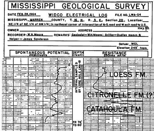
Figure 8.—Electrical log of Drill Hole LWA-S4 showing Loess silt.
