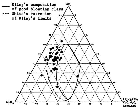
Figure 9.—Riley's diagram showing chemical analyses of 34 samples of previous testing that bloated below 2400°F.
