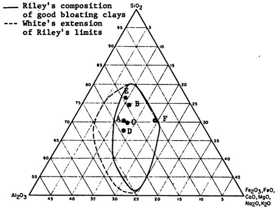
Figure 13.—Riley's diagram showing chemical analyses of alluvial clay [A=LWA-1 (1-22'); B=LWA-2 (1-12'); C=LWA-3 (1-11'); D=LWA-4 (1-8'); E=LWA-5 (0-19')] and Loess silt [F=LWA-18 (3-33')].
