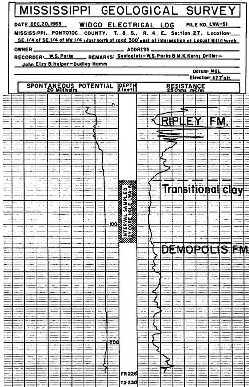
Figure 4.—Electrical log of Drill Hole LWA-S1 showing Ripley transitional clay.
