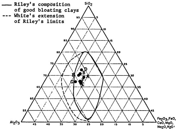
Figure 10.—Riley's diagram showing chemical analyses of Porters Creek clay [A=LWA-7 (6-34'); B=LWA-9 (7-52'); C=LWA-22 (2-32')], Zilpha clay [D=LWA-8 (18-55'); E=LWA-21 (12-52')] and Bucatunna clay [F=LWA-19 (20-39'); G=AF-1A (40-95')].
