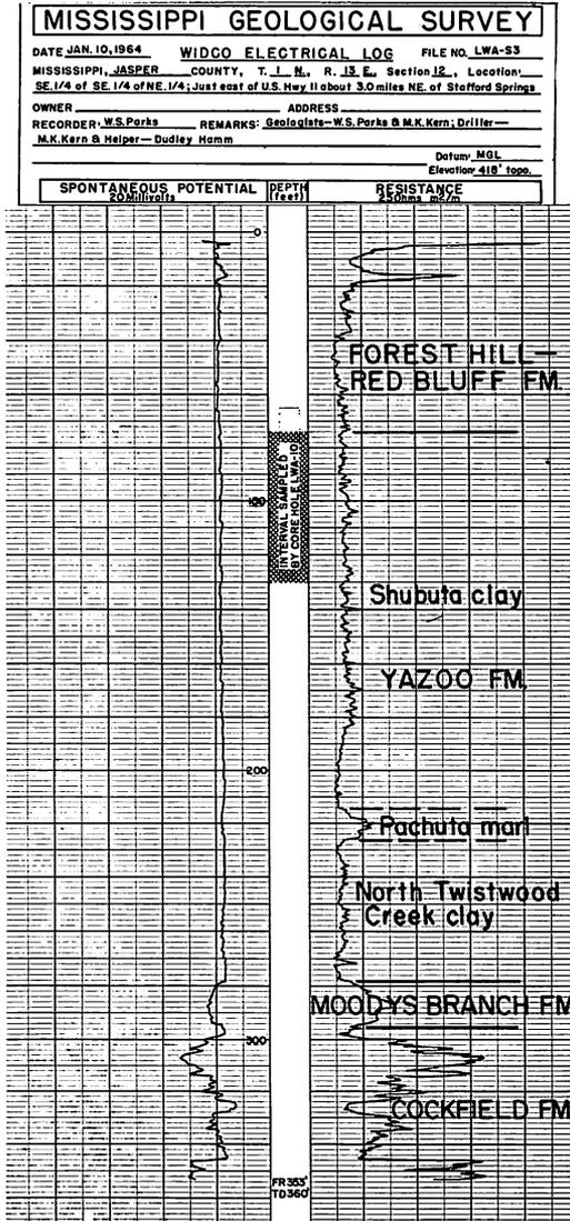
Figure 6.—Electrical log of Drill Hole LWA-53 showing Yazoo clay.
