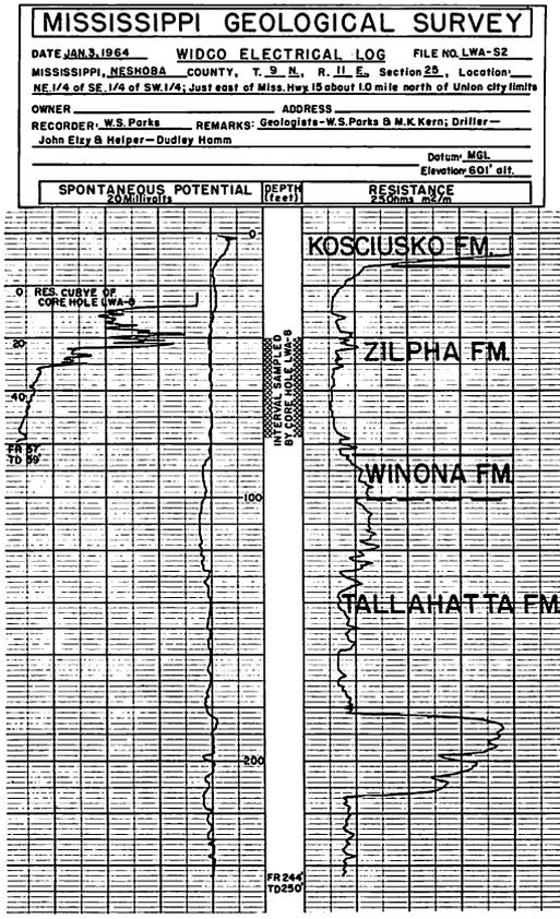
Figure 5.—Electrical log of Drill Hole LWA-S2 showing Zilpha clay.
