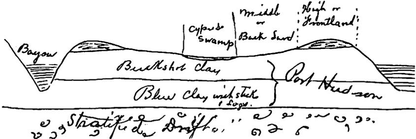
Figure 3.—Section in Mississippi Bottom, Showing Arrangement of Deposits.
