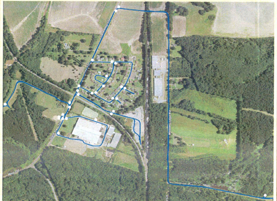
Figure 2: Outdoor air sampling locations collected in Eastern Heights and around the Facility by EPA's TAGA bus (mobile air sampling laboratory). The blue line is the 4.25 mile TAGA bus route. The white dots are the actual air sampling locations.
