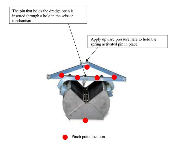
Refer to SWP HSP-3.15, "Manual Soil, Sediment and Waste Sampling" for additional safety information.
