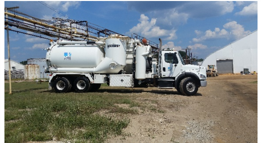
New "Guzzler" truck to assist in relocation of annular ring material
