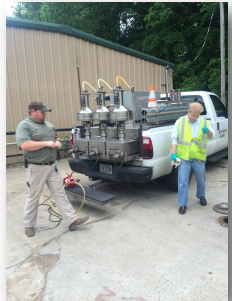
MDEQ's Dan Harper (right) and Andrew Villar, Mississippi Department of Agriculture and Commerce (left), measuring the amount of the fuel and water ratio in an Underground Storage Tank to determine how much had been pumped out.
