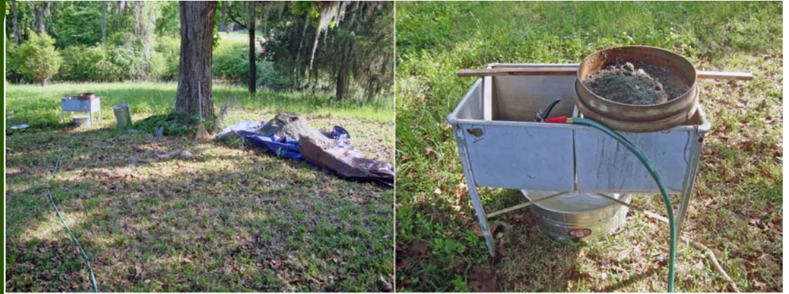
Figure 4. Left: Sieving operation and 3,000-pound pile of Moodys Branch Formation on tarps beneath shade tree. Right: Close-up view of sieve, vegetable washer, and washtub below to collect the fine fraction for re-sieving. Pictures were taken on April 26, 2014.
