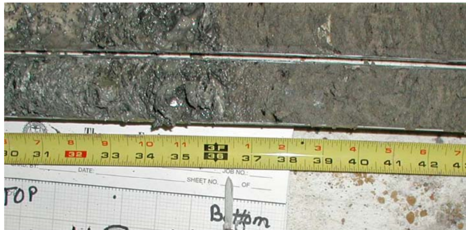
Figure 8. Core of the Imperial Palace property on Back Bay of Biloxi, showing the contact (at 3-foot mark) of fill (at left) and natural seafloor sediment (right).
