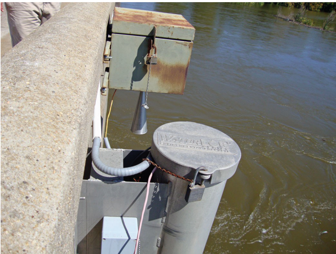
Figure 5. Radar gage measuring the river height from the Highway 80 bridge in Jackson. Picture was taken on September 7, 2011.
