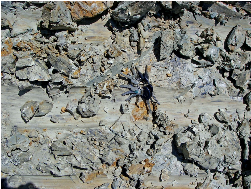
Figure 3. Unweathered Yazoo Clay in the bottom of excavation to remove slumped material along the east entrance for Dogwood Festival on Highway 25 in Flowood, Mississippi. Picture (digital DVD #59) taken on April 20, 2009.
