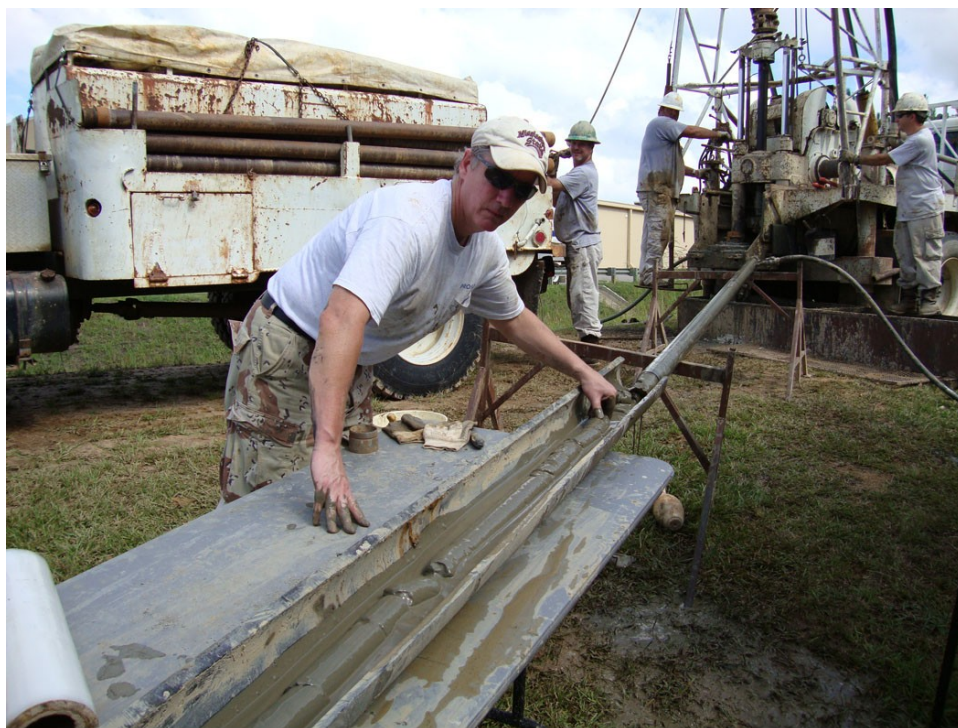
Figure 7. David Thompson positions the fifth core from 53-63 feet, which had a full ten feet of recovery. Jonathan McKinnon at upper left is attaching a new drill stem to the hoist cable, while Trey Magee (center) and Archie McKenzie (right) are operating the drill rig. Picture (digital DVD #63) taken on September 14, 2009.
