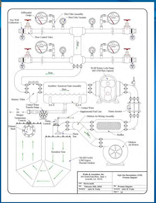
During the extraction process, the combined air and liquids are transferred to the HVR mobile treatment system. The liquids are separated from the airflow with a liquid scrubber/knock-out system and discharged into an internal storage tank for later disposal.
