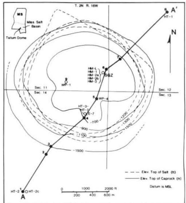
Figure 1. Well locations and structural contour map showing the configuration of the top of salt and caprock at Tatum Salt Dome, Mississippi. Location of geologic cross section A-A' is also shown. Modified from Taylor (1964) and Saunders (1988).
