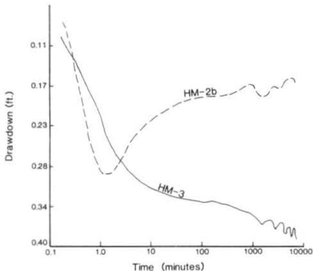
Figure 3. Semilogarithmic plot of drawdown data for pump tests of HM-2b screened in aquifer 2B and HM-3 screened in aquifer 3A. Pump discharge rates are 196.8 gallons per minute (GPM) and 192.7 GPM, respectively. From Fenske and Humphrey (1980).
