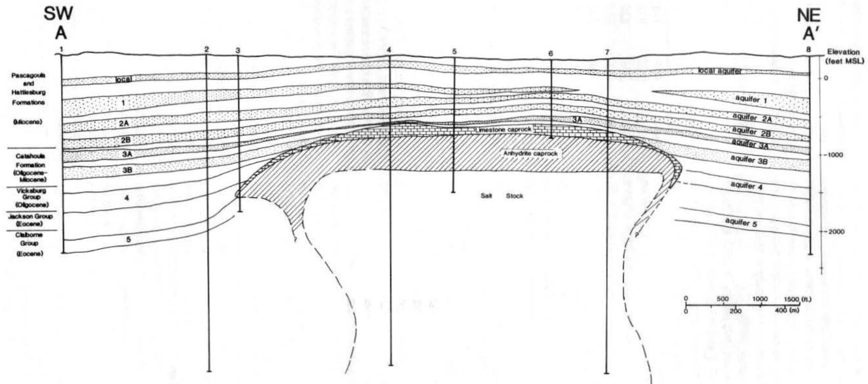
Figure 2. Geologic cross section A-A' through Tatum Salt Dome. Fresh-water aquifers are stippled. Modified from Taylor (1964).
