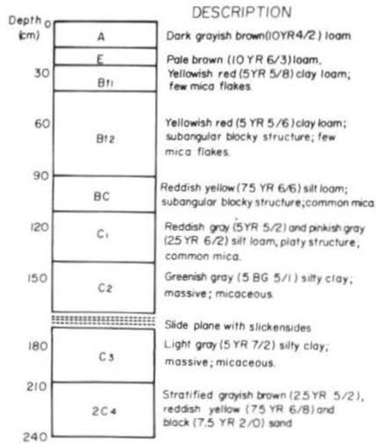
Figure 4. Soil profile of Choctaw County landslide site.
