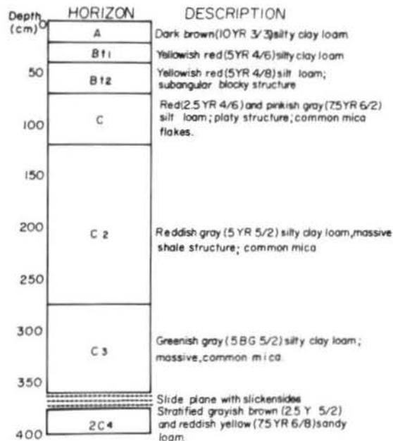
Figure 5. Soil profile of Winston County landslide site.
