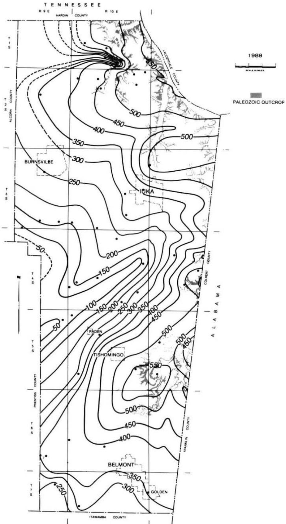
Figure 6. Contour map on the Paleozoic floor underlying Tishomingo County. Contour interval is 50 feet, datum mean sea level.
