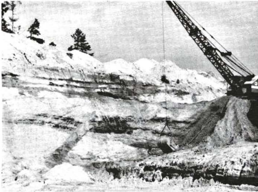
Figure 4. Gravel pit in Gordo Formation of Tuscaloosa Group in northeastern Itawamba County, Mississippi. Nearly twenty meters of chert gravel in quartz sand is exposed in the pit. Tuscaloosa gravels are the chief source of aggregate in the Tombigbee and Tennessee river systems in Mississippi and an important source for those beneath the loess and in southern Mississippi.
