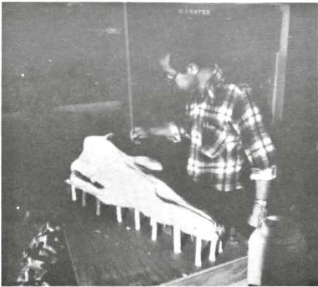
Figure 7. Applying layers of latex rubber to the dorsal side of the skull to form the upper mold.
