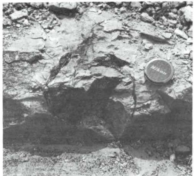
Figure 1. Oblique view of in situ, interconnected, tar-filled fissures in the Yazoo Clay at the Miss-Lite clay pit in Cynthia, Hinds County, Mississippi. Photograph was taken on July 18, 1985.
