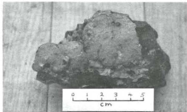
Figure 4. Tar fragment showing the lobate pillar morphology of the upper surface.
