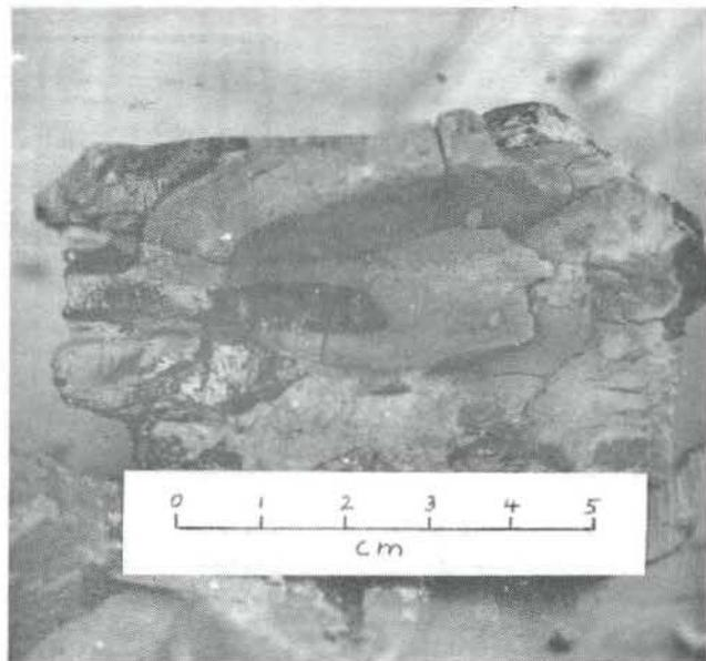
Figure 3. Tar fragment showing horizontal lenticular lobes penetrating the surrounding clay.
