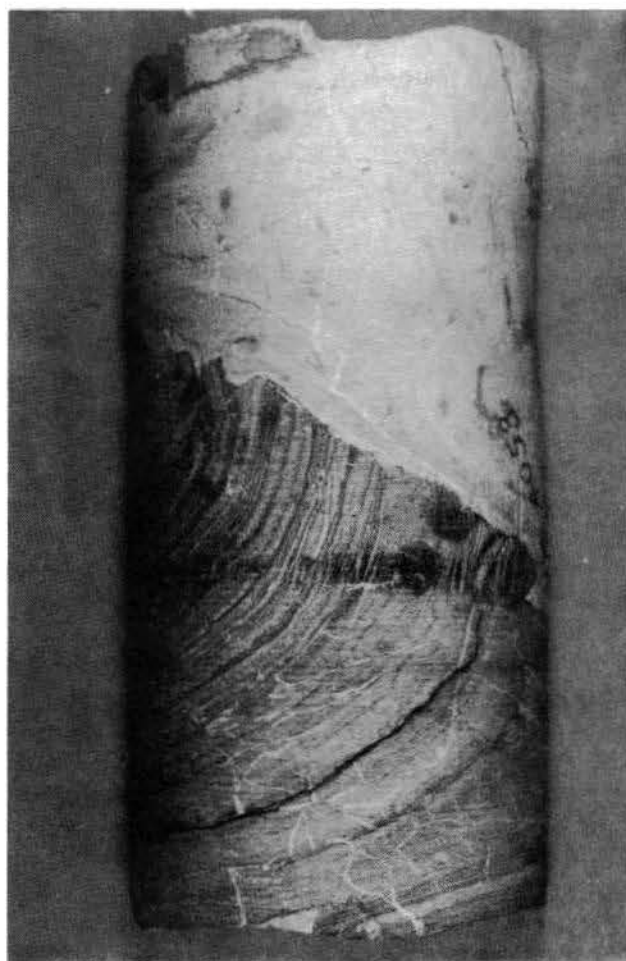
Figure 7. Cretaceous intrusive igneous rock, an intrusive phonolite, at lower contact with deformed, thinly-bedded Smackover Limestone from the Mississippi Valley Gas #1 Terry-Bell Unit in Section 18, T. 17 N., R. 9 W., Washington County, Mississippi, at 4053 feet. The 3.5-inch diameter core interval is from the bottom of Mississippi Office of Geology core box C-49.6.
