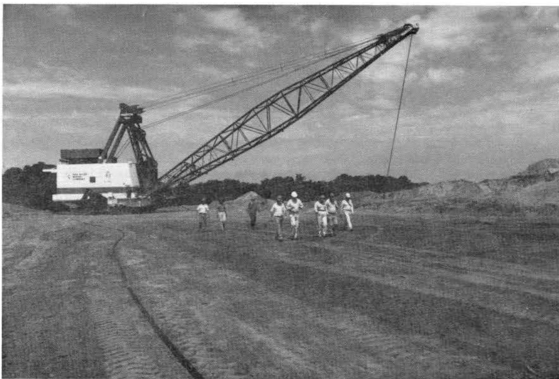
Figure 1. The large dragline for removing overburden at the Red River Mining Company's Oxbow Lignite Surface Mine near Coushatta, Louisiana, southeast of Shreveport. Photograph by Stanley C. Thieling, Mississippi Office of Geology, June 11, 1996.
