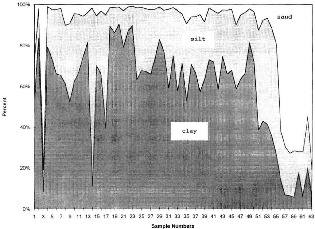
Figure 4. Percent clay, silt and sand for 63 samples from the Cockfield, Moodys Branch, and Yazoo formations. Sample 1 coincides with the top of the stratigraphic section, and sample 63 with bottom. Samples 1-55 are from the Yazoo Formation, 56-61 from the Moodys Branch Formation, and 62-63 from the Cockfield Formation.
