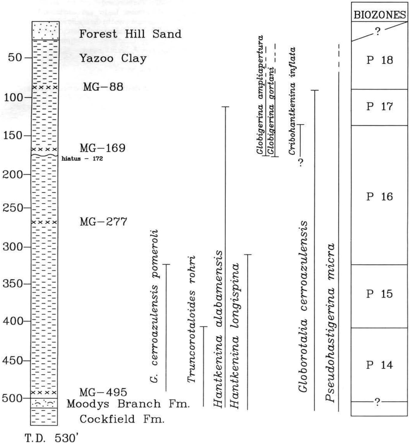
Figure 1. Columnar section of the Mossy Grove core showing ranges of selected planktonic foraminifera and the assigned biozones. Bentonites are identified on the section by the "MG" designation. Biozone definitions are after Berggren and Miller (1988).
