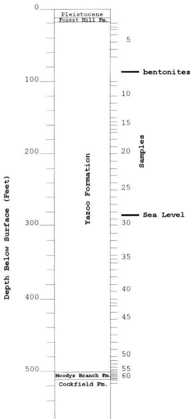
Figure 2. Generalized stratigraphic section in Mossy Grove Core #1 showing formations, depth (in feet) relative to land surface, samples used in this study, and stratigraphic position of bentonite layers (modified from Dockery and others, 1991).
