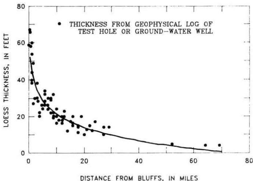
Figure 2. Relation of total loess thicknesses determined from geophysical logs to distances of test holes and wells from the Mississippi River bluffs in the Memphis, Tennessee - northern Mississippi area.
