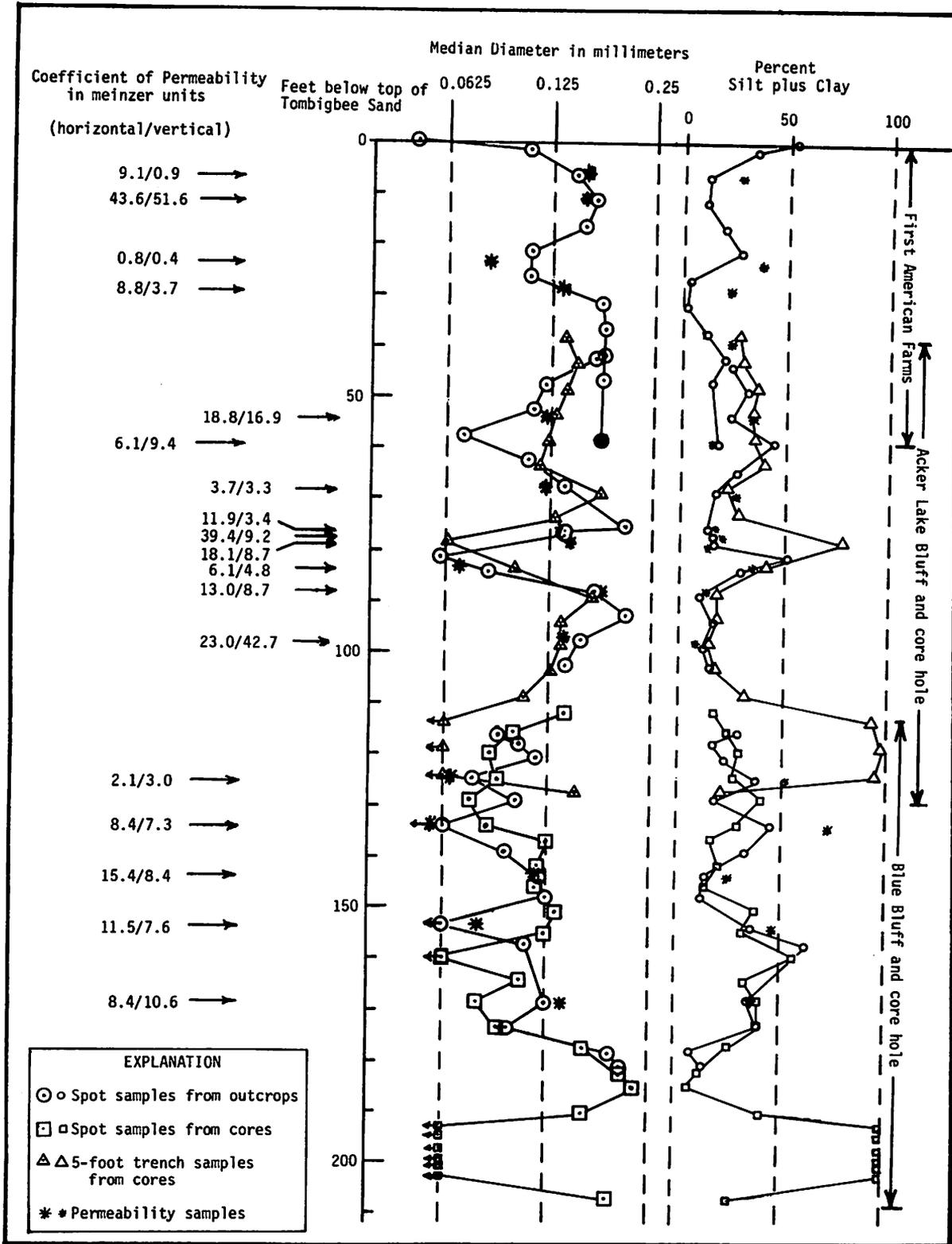
Fig. 9. Diagram showing value of sedimentary parameters and their projected positions on the composite stratigraphic section of the Tombigbee Sand.
