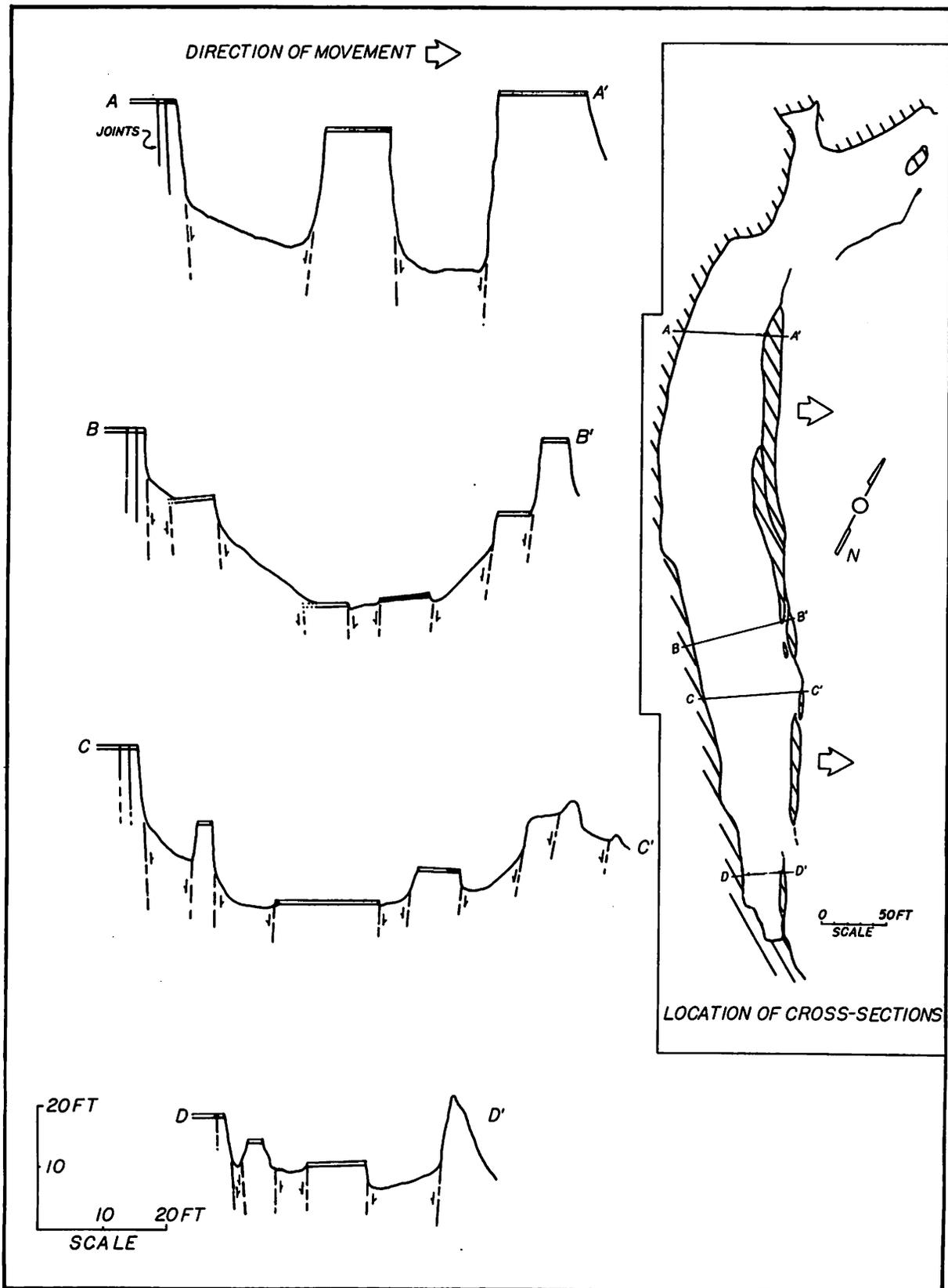
Fig. 4. Diagrammatic cross section showing surface profiles and major fractures in the northern graben area.
