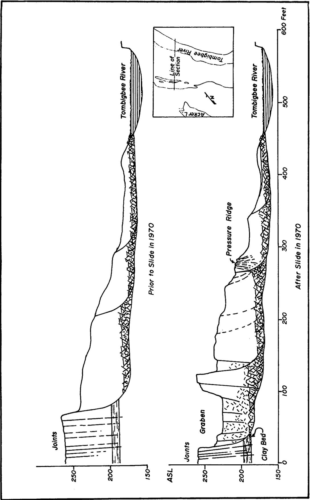
Fig. 12. Diagrammatic cross sections showing postulated conditions before and after 1970 slide.
