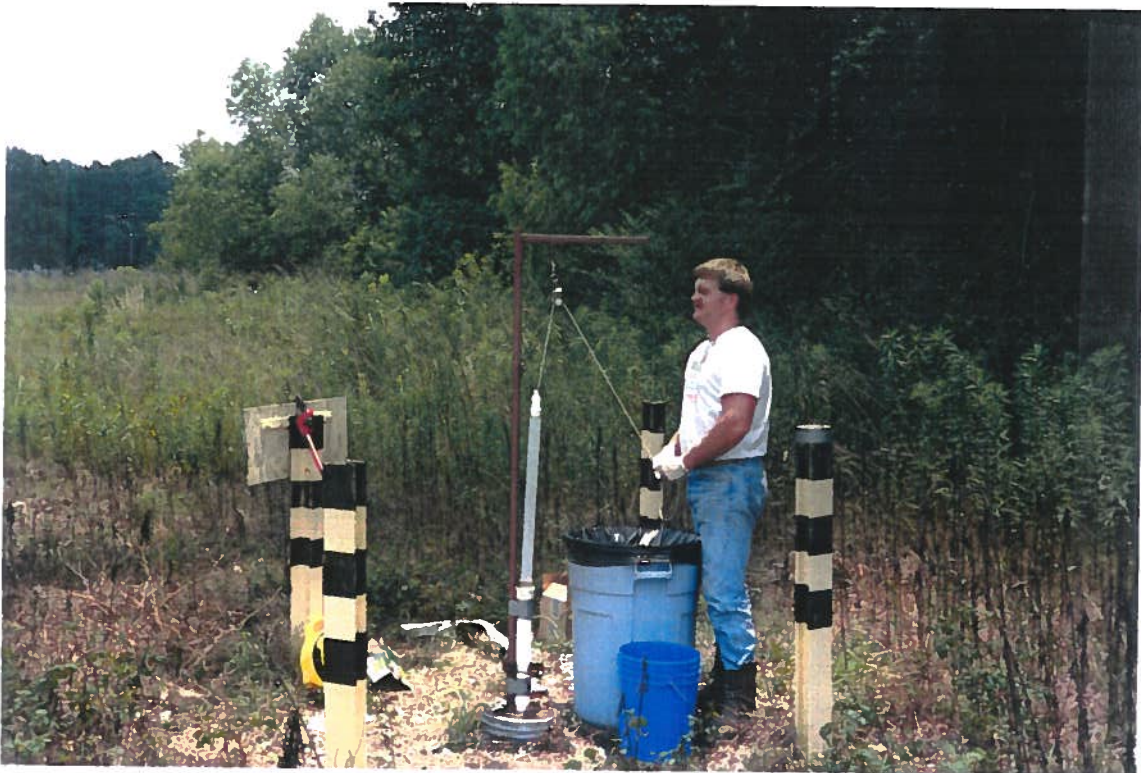
Photo # 24 Roll # 2 Frame #: 1 Date: 6/25/92 Subject: Purging monitoring well B-1, in the "back forty" portion of site property. Preparing for Sample HI-MW-B1
