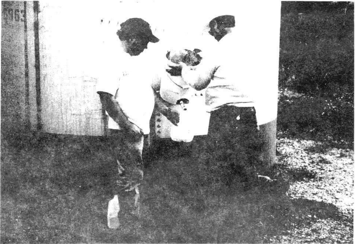
Figure 7. Transfer of brine sample into sample collection bottle.
